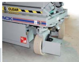
90° steering (zero inside turning radius)
